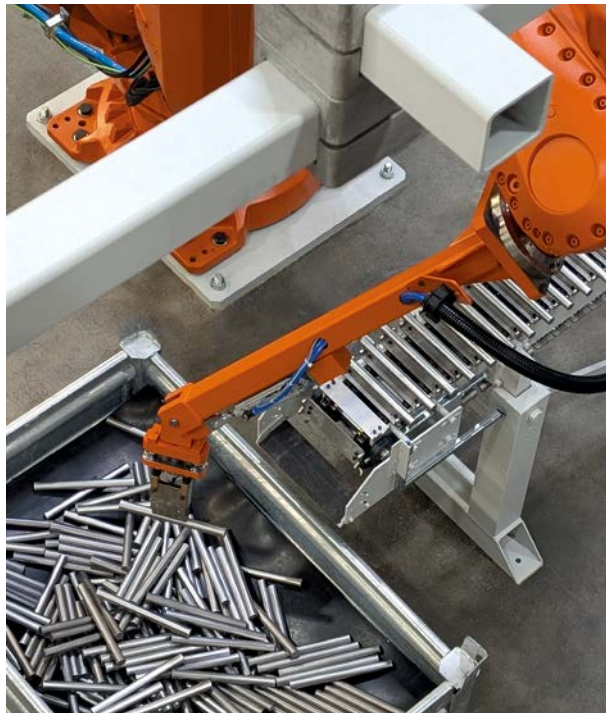
The position and orientation of accessible parts in the container are automatically detected.
