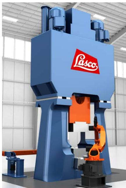
Automated forging hammer HO-U 160 in schematic representation.
