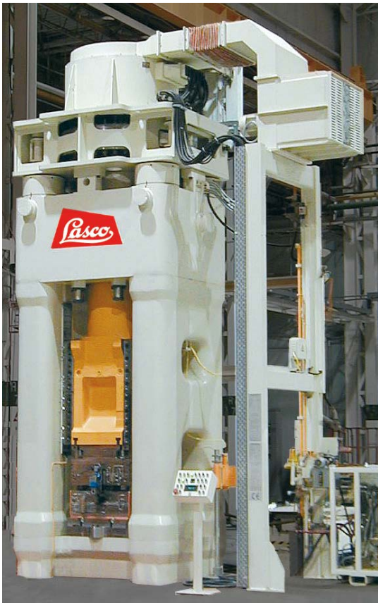
Screw presses (Pic.: LASCO SPR 2000) can be controlled very precisely due to the exact dosing of the forming energy and are therefore ideally suited for the forming of demanding materials such as aluminum.
