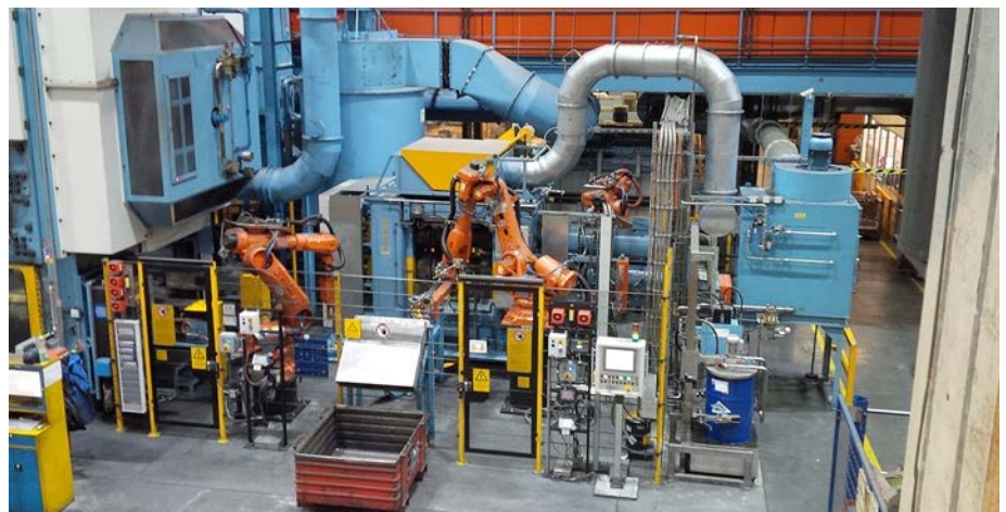
The production line „AMP58” with integrated LASCO forging roll at the Hirschvogel Aluminium GmbH (HAG) in Marksuhl (Thuringia/Germany).
