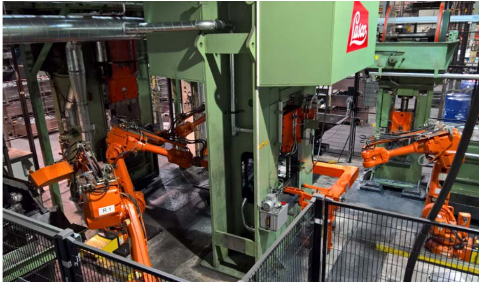
High-quality Fiskars™ axe blades (shown left) are produced fully automatically (see production line above) – in Billnäs/Finland. LASCO integrated existing and new line components to make up an efficient, fully automatic production line.
