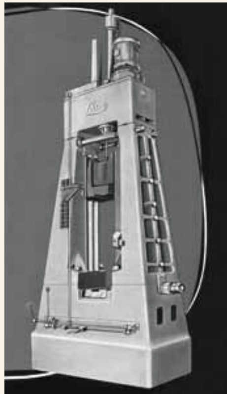
First electro oil-hydraulic die forging hammer worldwide – LASCO patent no. 974854 dd. 1951
