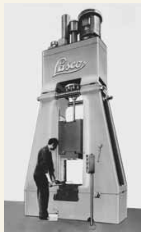
Electro oil-hydraulic LASCO die forging hammer KH/KGK
