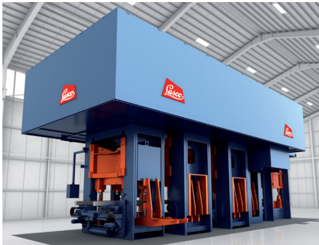
Press line consisting of five deep-drawing presses
