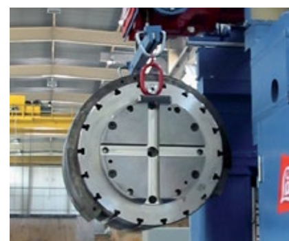
Roller change device: A roller can be exchanged in less than 10 minutes
