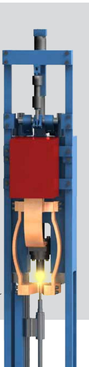
Upsetting unit of an electro-upsetter type EV
