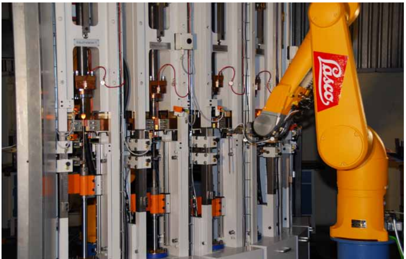
Electro-upsetting line EV 16 with 6 upsetting units
