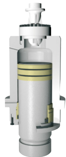
Press cylinder of a LASCO MXP (schematic view)
