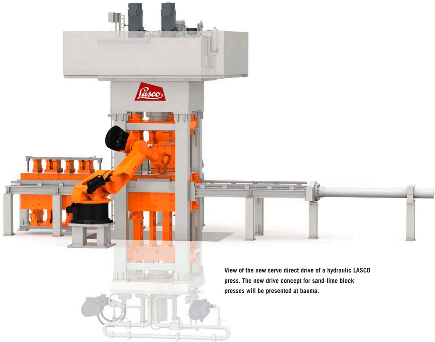
View of the new servo direct drive of a hydraulic LASCOPress. The new drive concept for sand-lime block presses will be presented at bauma.
